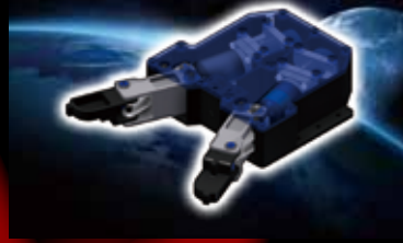
Robotic Hand for Extravehicular Activity in Space
