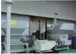
Grinding sludge is solidified, and waste converted into steel materials (valuable item)
