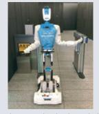
The thermometric robot keeps its left arm up when a body temperature exceeds a certain amount
