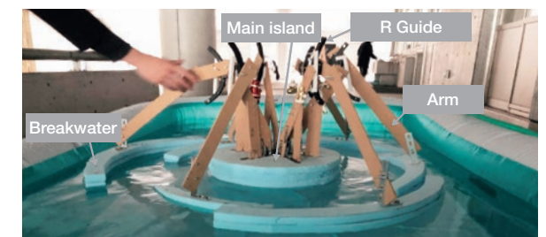
The R Guide protects the island by absorbing wave motion
