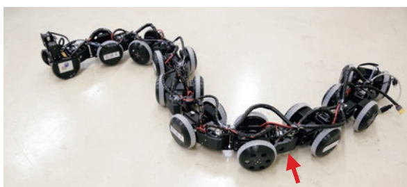
The T2 Snake-3 features a SEED MS on the side of each joint (indicated by the arrow)
