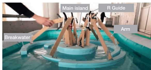
The R Guide protects the island by absorbing wave motion
