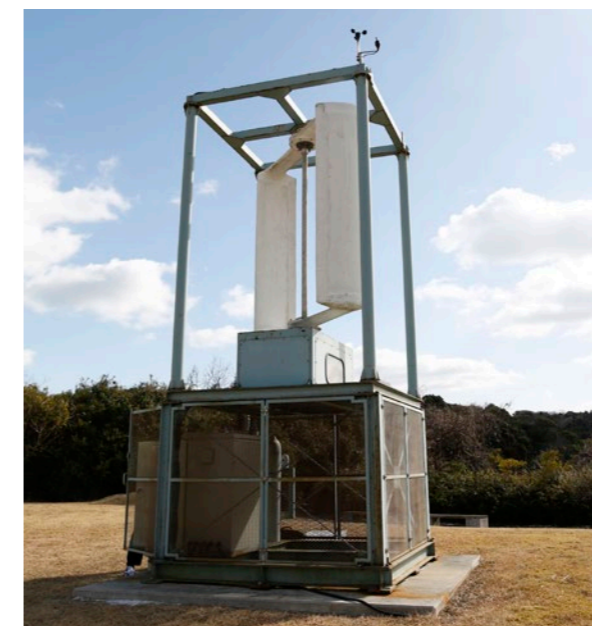
Improved small wind turbine on the institute's grounds
