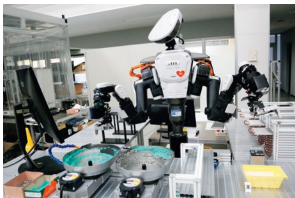
NEXTAGE® using the cameras on its left and right hands to identify the spatial relationships between objects as it works
