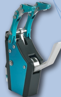
Robot Hand Model TRX 2015 Using a miniature ball screw allowed for a compact design and increased gripping power.
