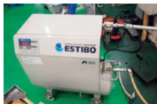
Electric booster compressor
