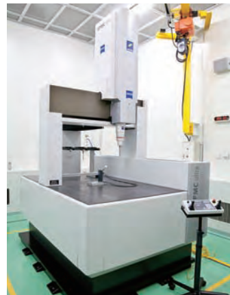
Seismically isolated 3D measuring device.
