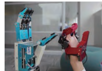
The movements of JAXA's robotic hand (at left) mirror those of a robotic glove.
