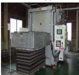
▲ Vacuum carburizing furnace at the YAMAGUCHI Plant
