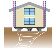
The dotted line shows the vibration with seismic isolation.
