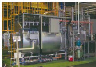
Drip-feed carburizing furnace installed in March 2007 at the YAMAGATA Plant
