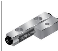
Cross-Roller Guide Model VRG This product achieves light, smooth motion by not recirculating the rolling elements. THK's proprietary rack and pinion mechanism prevents cage misalignment and provides stable motion.
